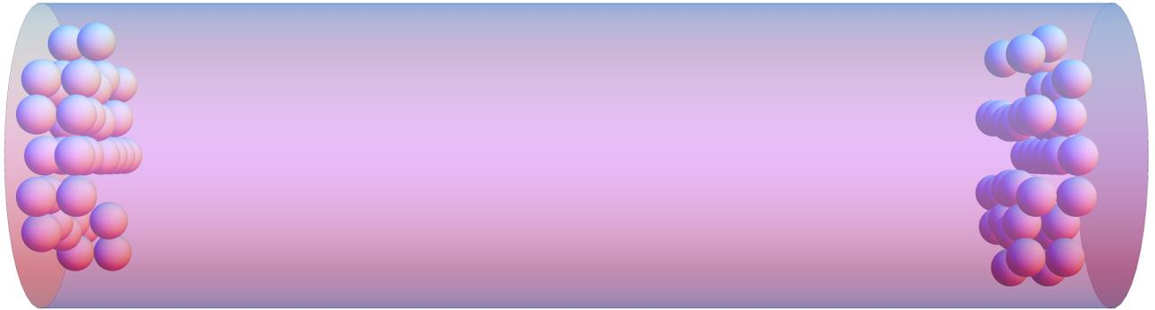
**Figure 2.4** A depiction of the two-section broken glass detector is shown above. Rendering the many thousands of glass spheres positioned within the detector would be impractical, so only a few representative spheres are shown and the size of the detector is greatly reduced.
