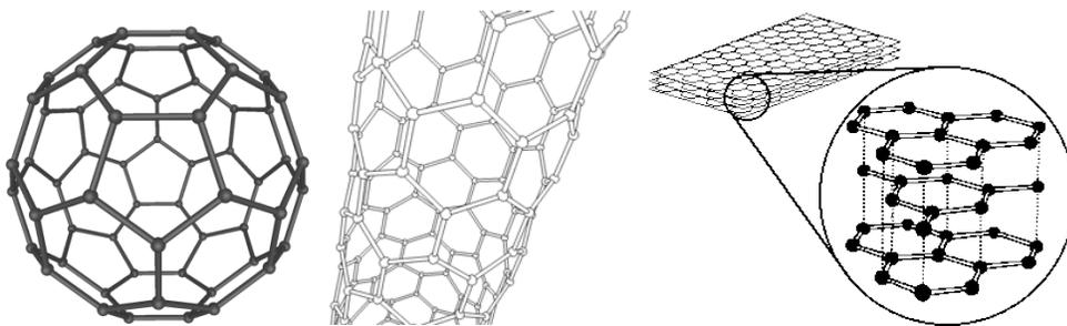
Figure 1.1 Left: Buckyball, Center: Carbon nanotube, Right: Graphite
