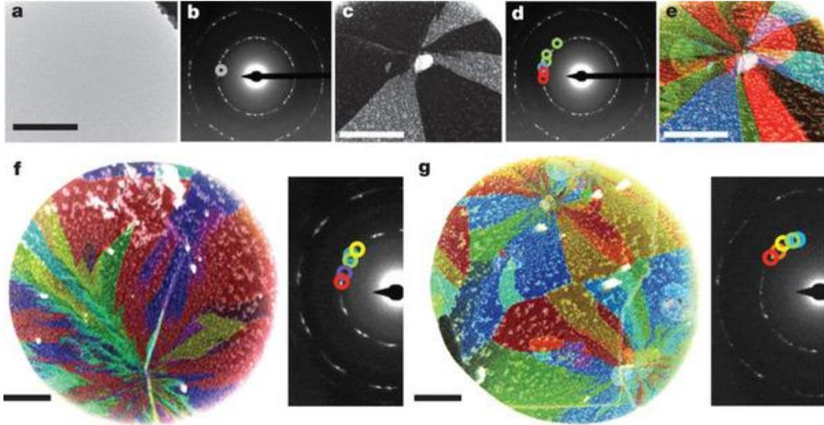
**Figure 1.2 Grain Boundaries on Graphene [3] a-g: TEM images of grain boundaries, scale bars 500nm.**
