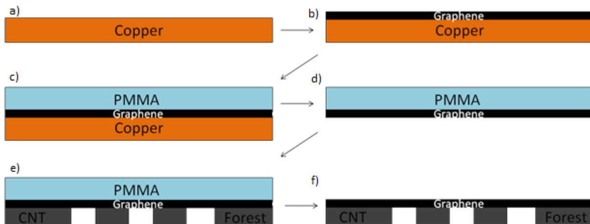
Figure 2.7 a) The copper foil is treated and prepped for graphene growth, b) graphene is grown by chemical vapor deposition, c) PMMA is spun on the graphene and copper foil, d) The copper foil is etched away using Sodium Persulfate, e) The PMMA/graphene membrane is transferred to the carbon nanotube support, f) The PMMA is removed with 1165 leaving a graphene suspended over holes in the carbon nanotube forest
