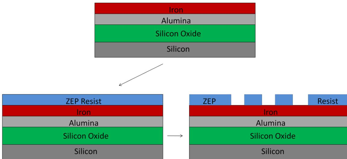
Figure 2.3 Left: ZEP Resist is spun on the iron layer, Right: The resist is patterned by electron beam lithography and developed away leaving a pattern in the resist
