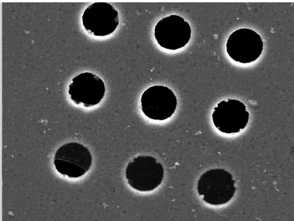
Figure 3.5 SEM image of an array from figure 3.4. Only three of the nine holes were covered with one being only partially covered.
