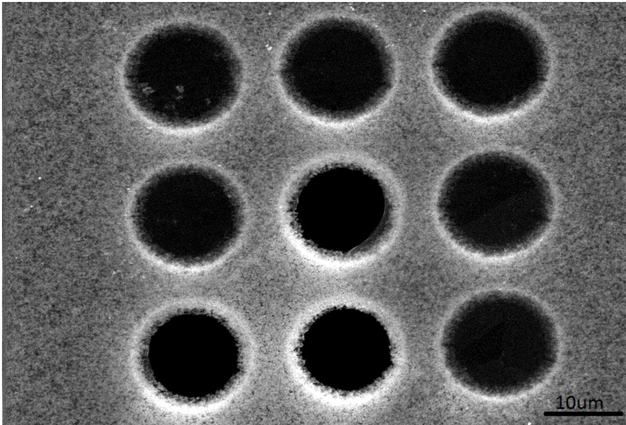
**Figure 3.7 SEM image of graphene suspended over 10um holes in a carbon nanotube forest. The center and two lower left holes are not covered with graphene while the remaining six are. The copper grain structure can be easily observed in the lower right graphene membrane.**
