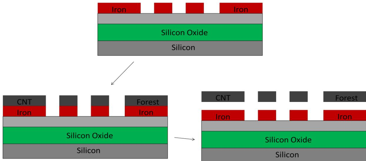
**Figure 2.6 Left: A carbon nanotube forest is grown on the iron catalyst, Right: The CNT forest is released from the sample during infiltration**
