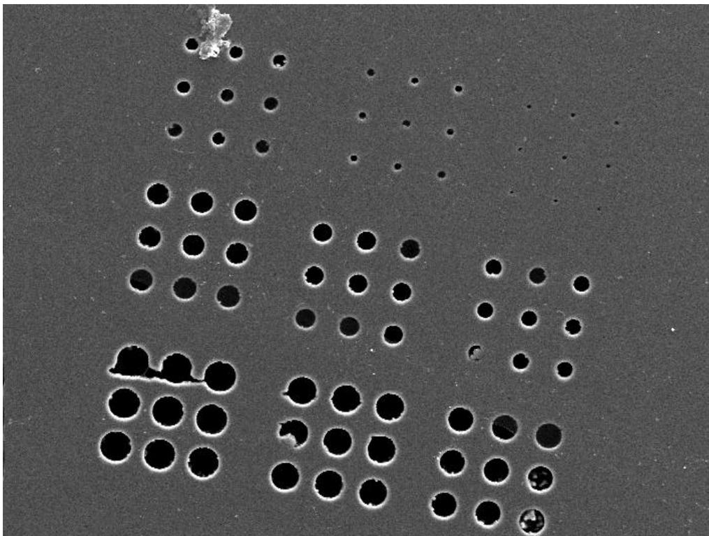
Figure 3.4 SEM image of successful graphene transfer. Only 11 of the 81 holes were successfully covered with graphene.
