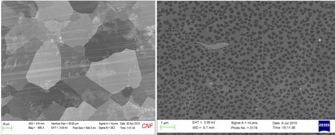
**Figure 1.3 Left: SEM image of copper grain boundaries from a single copper foil, Right: SEM image of graphene grains on a single copper grain**
