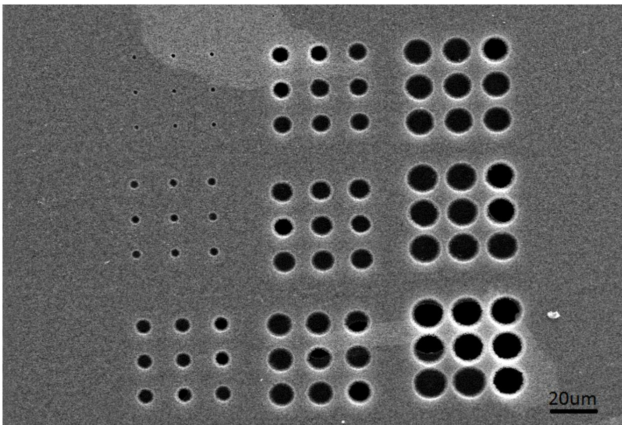
Figure 3.3 SEM image of holes in a carbon nanotube forest. The holes range in size from 2-20um.
