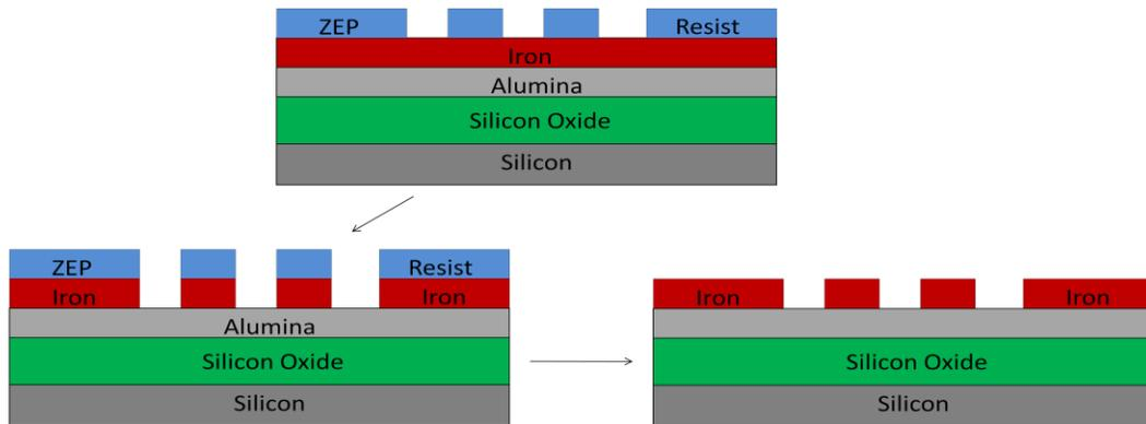
Figure 2.4 Left: Lithography pattern transferred to the iron by etching in HCl, Right: The resist is removed using 1165
