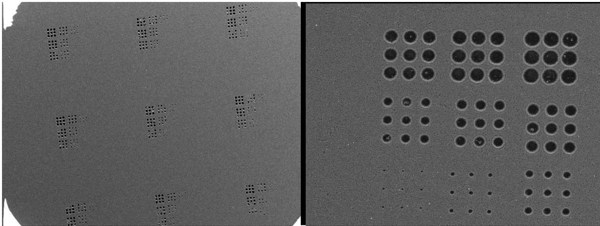
Figure 2.2 Left: SEM image of nine large arrays, Right: Nine arrays of nine circles ranging form 1-10 um
