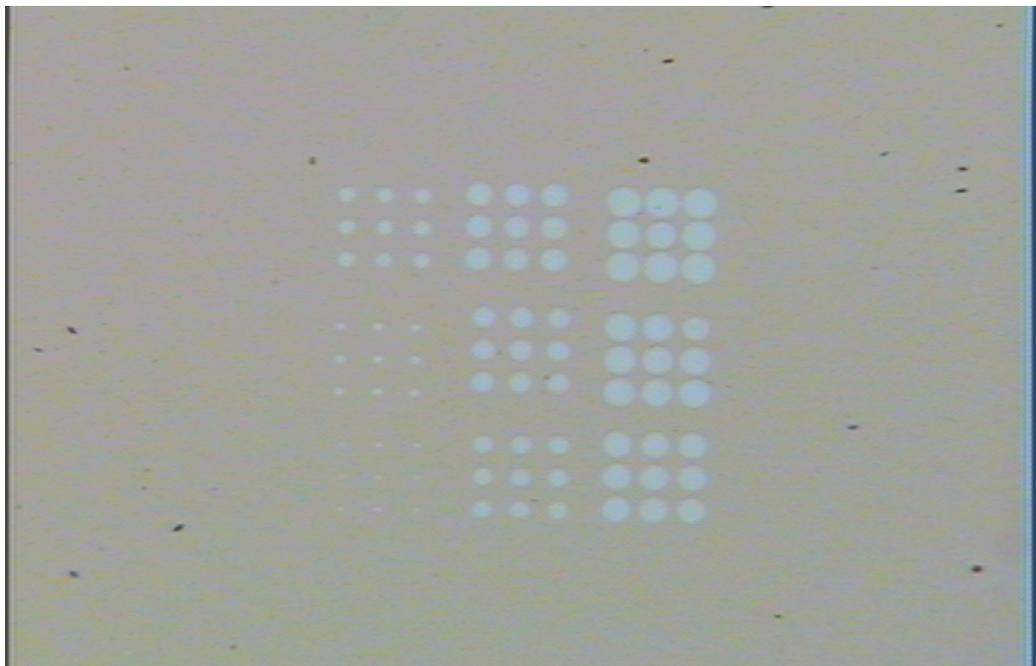
Figure 2.5 Light microscope image of lithography pattern transferred to the iron layer
