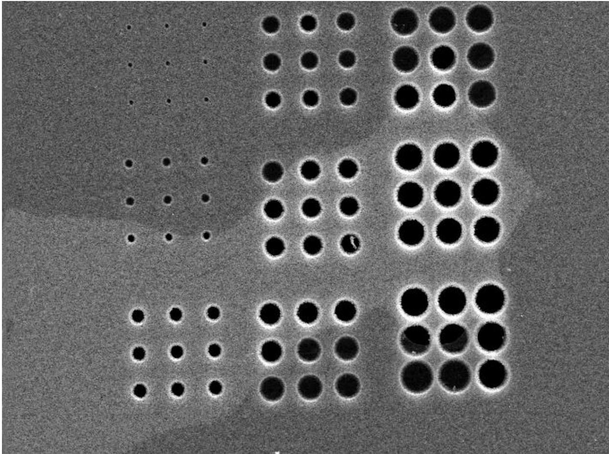
**Figure 3.6 SEM image of plasma cleaned sample. Darker contrast areas indicate successful graphene transfer. In lighter areas no graphene was on the surface.**
