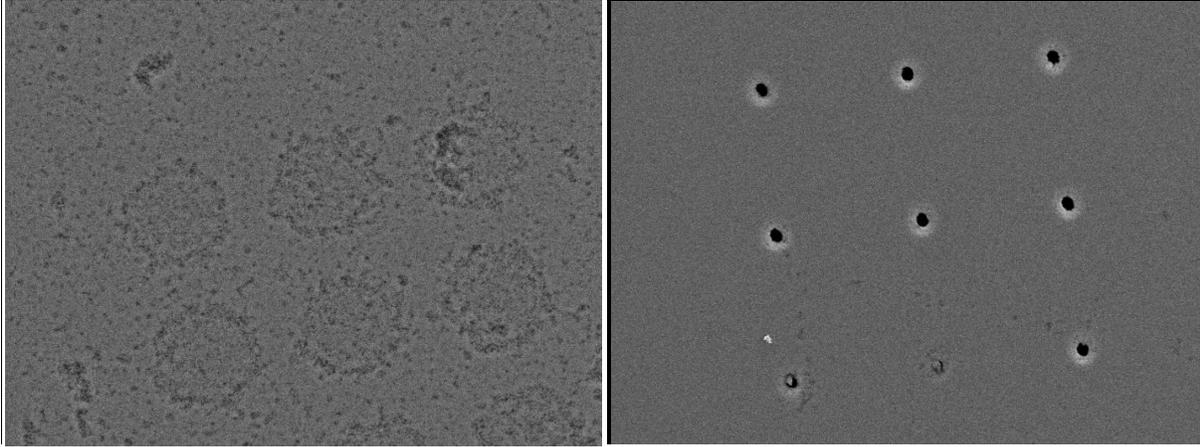
**Figure 3.2 Left: SEM image of carbon nanotube forest after release and before sonication. The holes are covered in a carbon floor layer. Right: SEM image of carbon nanotube forest after sonication. Carbon floor layer has been removed and holes extend through the whole sample.**
