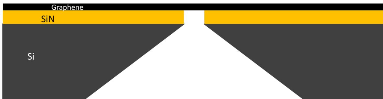
**Figure 1.4 Tapered edges of a silicon wafer having undergone an etching process. Also, an additional layer such as  $\text{SiN}$  makes fabrication and alignment considerably more difficult.**
