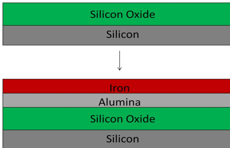
**Figure 2.1 30nm of Alumina and 7nm of iron are deposited on a silicon wafer**
