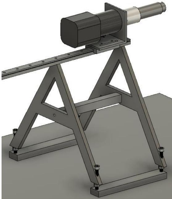
*Figure 4 The final design. The rail is bolted to the A-frame. The frame is supported by screws which allow for the height to be adjusted for perfect connection between the motor and the micrometer knob.*
