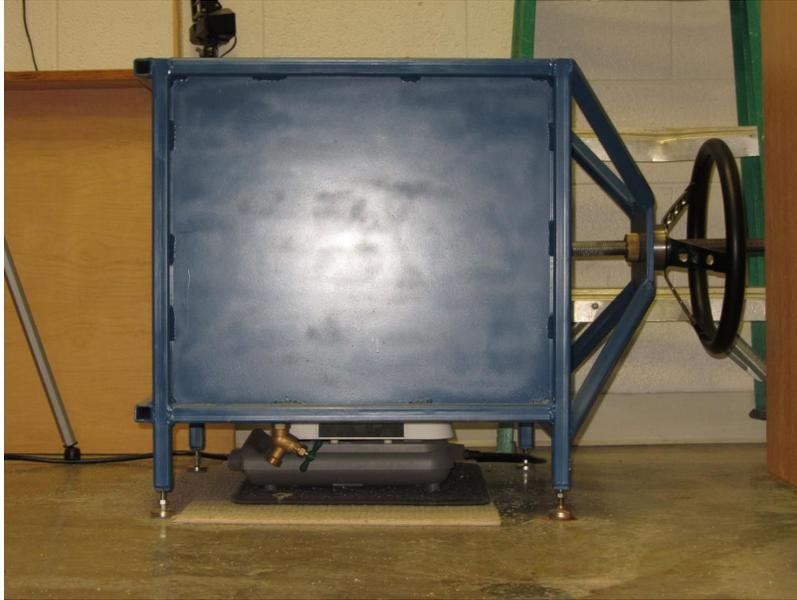
*Figure 1: Experimental Apparatus, with hot plate and moveable wall*
