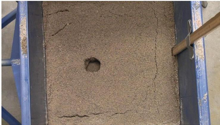
*Figure 7: Initial collapse 40 minutes into Experiment 3.*
