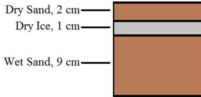
*Figure 2: Experiment 1, model with one thin layer of dry ice*
