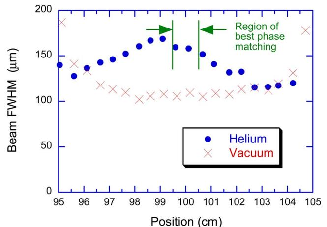
Fig. 3. (Color online) Diameter of the laser as it exits from the gas cell, either filled with 80 Torr helium or evacuated. The best focus in the absence of gas occurs 100 cm after the focusing mirror.
