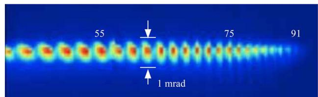
Fig. 1. (Color online) High harmonics produced in 80 Torr helium dispersed by a grating onto a detector.
