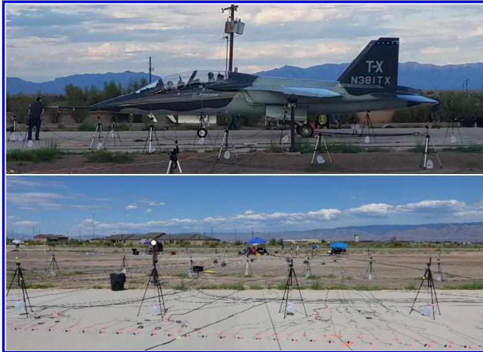
**Figure 1: T-7A “Red Hawk” tied down at Holloman Air Force Base (above). View from the aircraft looking out toward far-field microphones (below).**
