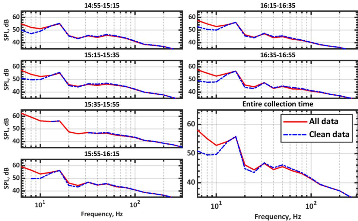
*Figure 6. Wind noise reduction applied to the spectral data shown in Figure 5. Results are shown for 20-minute intervals, along with results for the entire collection period.*
