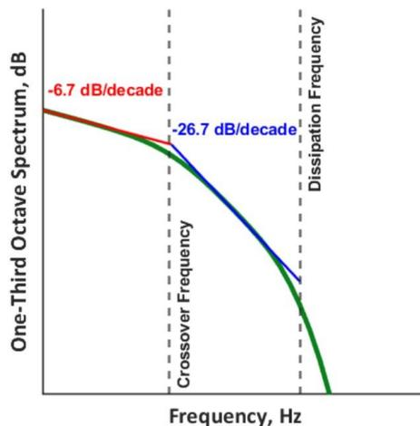
**Figure 1. Visualization of spectral wind noise characteristics in the inertial subrange. Above the crossover frequency and before the dissipation range, the characteristic slope of wind noise is -26.7 dB per decade.**
