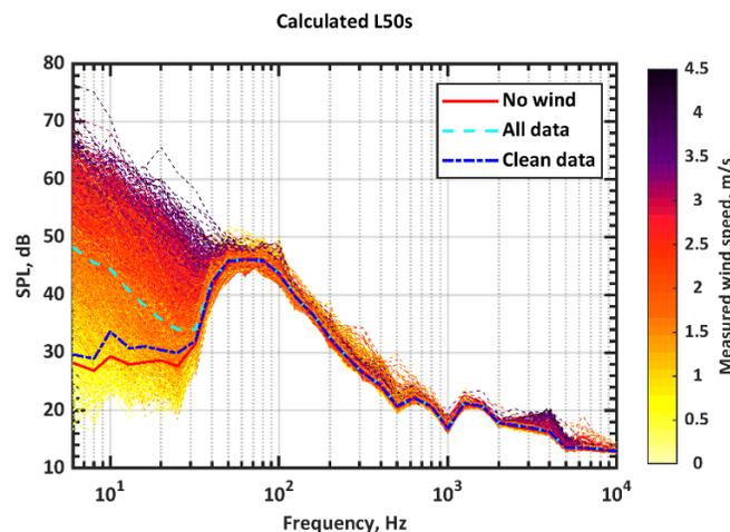
**Figure 2. Wind contamination reduction results for a constant brown noise source. Below 50 Hz measured levels are primarily caused by wind contamination. The reduction method median level approximates the median level when wind speeds of 0 m/s were measured, indicating that the method is able to correctly classify frequencies where spectral data are a product of wind noise rather than acoustic noise.**
