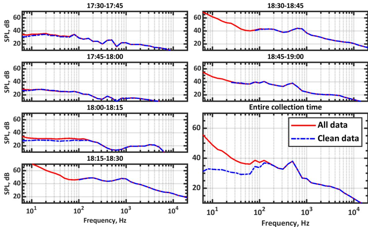
**Figure 4.** Wind noise reduction applied to the spectral data shown in Figure 3. Results are shown for 15-minute intervals, along with results for the entire collection period. For the clean data average, frequencies that were contaminated for more than 75% of the measurement period are omitted.
