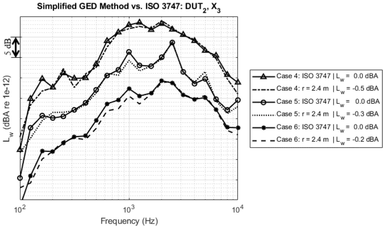
Figure 4. The sound power of DUT<sub>2</sub> measured at a distance of 2.4 m in Case 4, 5, and 6 using the simplified GED method compared to the sound power measured using ISO 3747.
