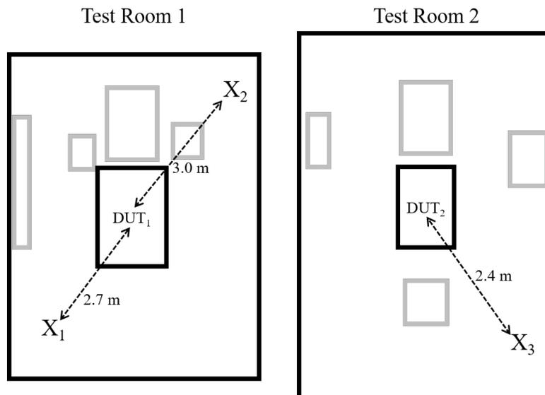
Figure 1. The layout of Test Rooms 1 and 2 showing DUT locations, sensor locations and distances, and support equipment (gray boxes) present for the measurement.
