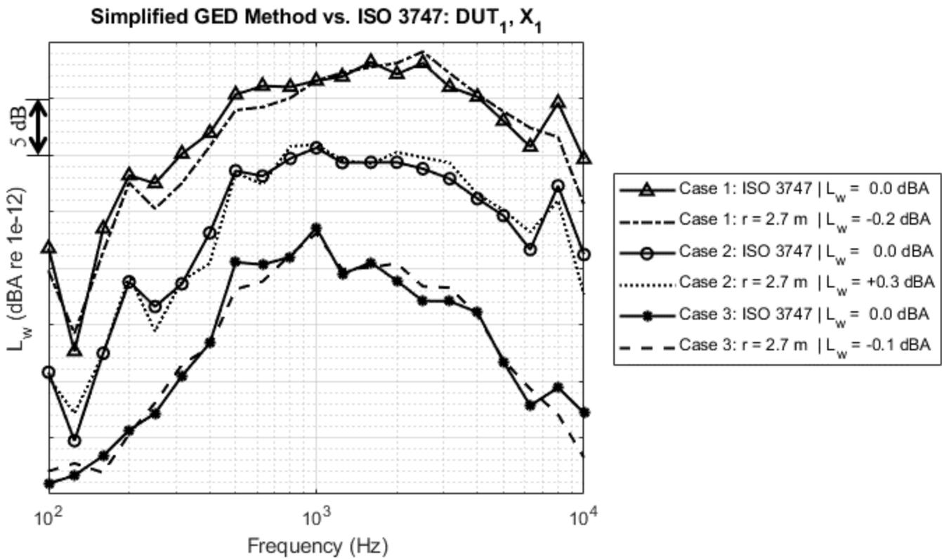
Figure 2. The sound power of DUT<sub>1</sub> measured at a distance of 2.7 m in Case 1, 2, and 3 using the simplified GED method compared to the sound power measured using ISO 3747.
