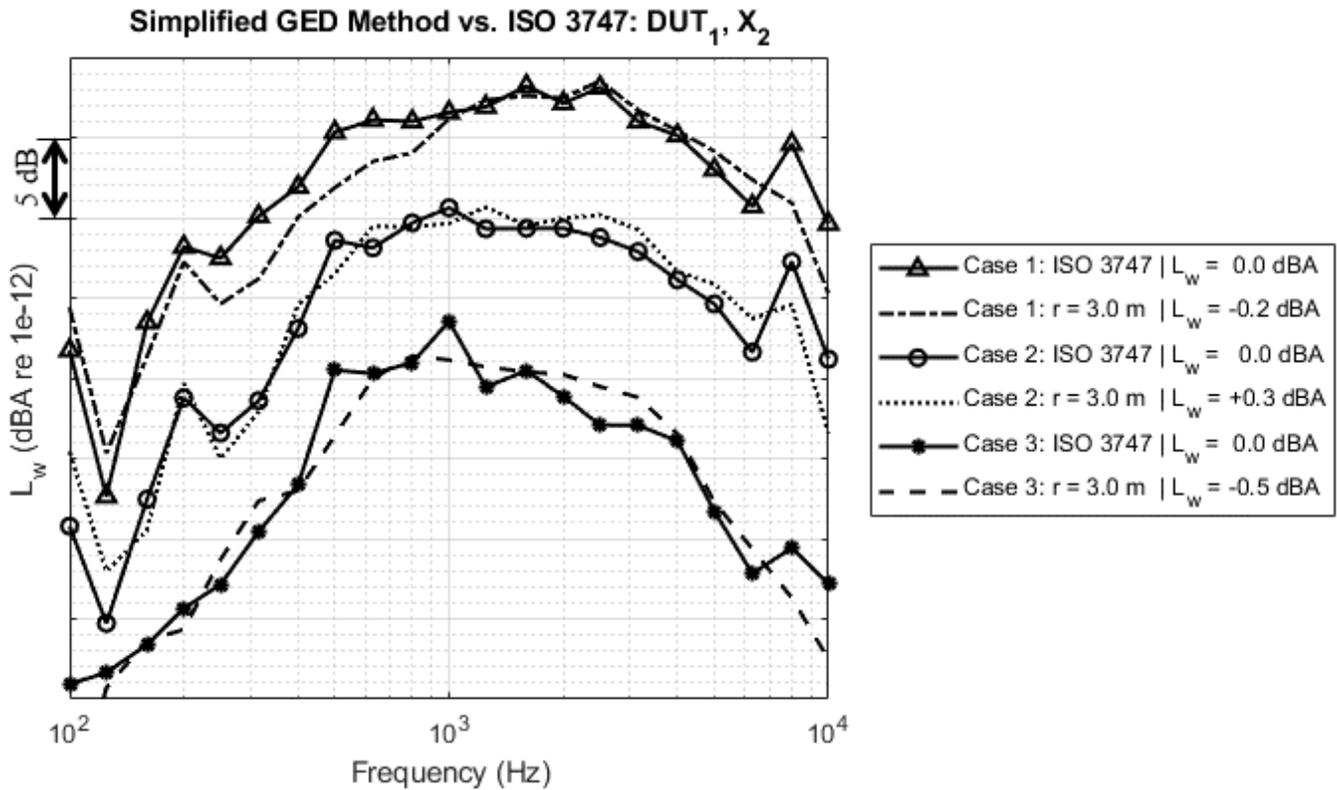
Figure 3. The sound power of DUT<sub>1</sub> measured at a distance of 3.0 m in Case 1, 2, and 3 using the simplified GED method compared to the sound power measured using ISO 3747.
