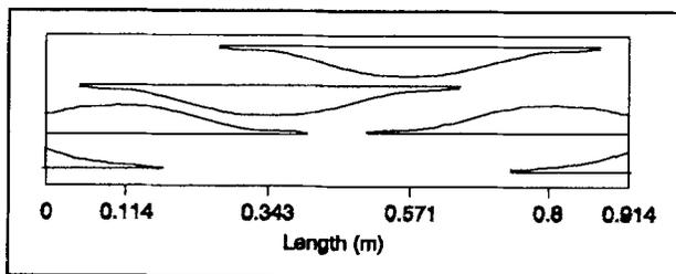
**Figure 2.** Schematic showing the layout of the shaped sensors on the clamped-clamped beam.
