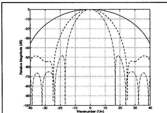
**Figure 1.** Wavenumber response of shaped sensors. Sensor lengths shown are: \_\_\_\_\_ 0.3 m; - - - 0.6 m; - . - . 1.0 m;
