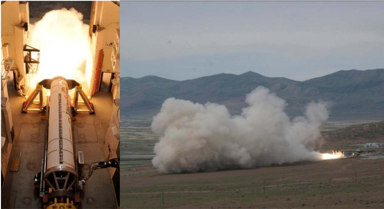
*Fig. 2 - GMD stage 1 Orion-50 horizontal static firing observed from above the test cell (left) and from the T-97 viewing area (right).*
