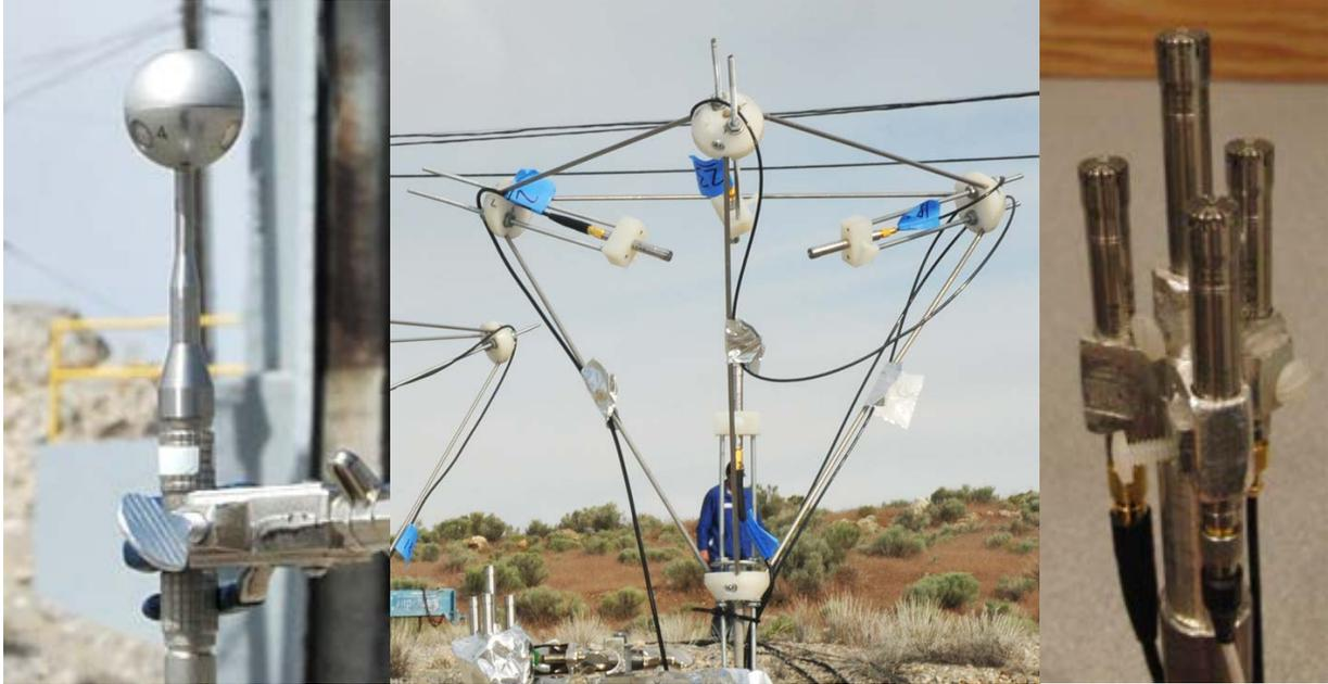
*Fig. 1 – Microphone configurations evaluated in the study. Left: spherical probe, center: external frame probe, right: parallel axis probes.*
