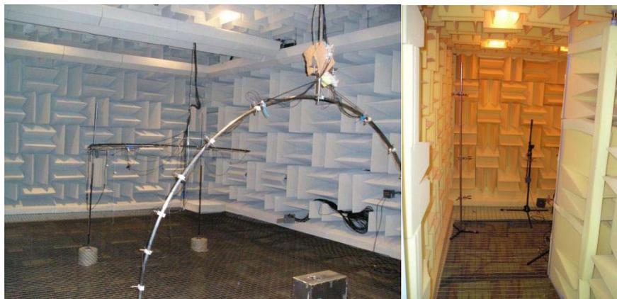
**Figure 3.** Left: BYU fully anechoic chamber renovated with perforated metal wedges. Right: A smaller, recently built fully anechoic chamber with foam wedges that can be used for ultrasonic measurements.
