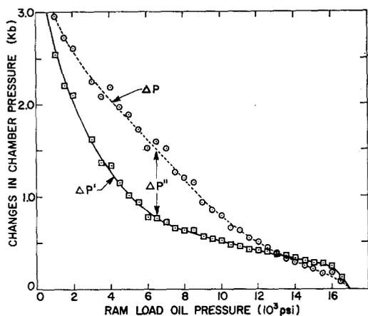
Fig. 5. Magnitude of chamber pressure changes resulting from equal sized step decreases at different load pressures—( $\Delta P'$ ), during time load is decreasing and ( $\Delta P$ ), total change before approximate equilibrium is reached. ( $\Delta P''$ ) represents nonequilibrium stresses immediately following a decrease in load pressure.
